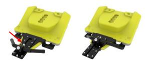
The hand grip can also be rotated in 3 different positions indicated by a letter (A-C). Pull the white button indicated by the red arrow in the picture below, adjust the angle and push the button to lock.
