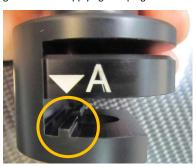
Turn the top portion of the handhold clockwise to clamp, see marking on top of the device.
