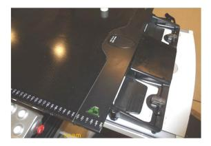
Insert the extension to the interface couch under a slight inclination angle.
