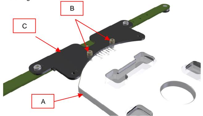
Screw the adapter plate onto the base plate using the M6x12 hex cap screws and Allen wrench 5 mm.
