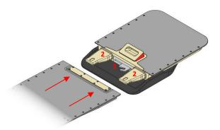
3. Slide the extension towards the base. By sliding the extension towards the base, the latch plate (3) will turn into the locked position. The release handle (1) – which is connected with the locking pin – will fall down into the locking position.
