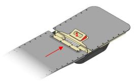
4. When the handle surface is flush with the top surface of the couch (the red unlock sign is not visible), and when there is a small seam of +/- 1 mm between the couch and the extension, then the couch extension is correctly secured to the couch base.
