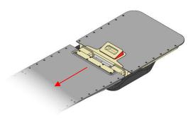
3. When reaching the stop (second safety mechanism), lift the extension slightly.
