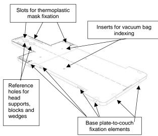
This base plate has a cut-out with a removable bottom part which makes it compatible with the HexaPOD™ evo RT system. When removing the bottom part, the iBeam holes are not covered by the base plate so the HexaPOD frame can be attached to the iBeam table.
