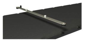
To position this 2-pin bar on such a couch, gently push the bar with its two indexing elements into a set of couch cut-outs and rotate the lever of the moving element into the 'locked' state. The bar itself should now be flat on the surface of the couch. Always make sure that the bar is well positioned on the couch before indexing the other hardware to the 2-pin bar.
