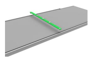
To position this 2-pin bar on such a couch, gently push the bar into the couch cut-outs. The bar itself should be flat on the surface of the couch. The 2-pin bar will be able to slide in a longitudinal direction. Always make sure that the bar is well positioned on the couch before indexing other hardware to the 2-pin bar.
