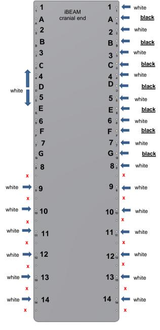
The standard setup with two white pins is usable on 14 locations. It is preferred to try and use these first.
