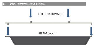
Orfit hardware is mounted on the 2-pin bar by simply pushing it over the 2 middle pins.
